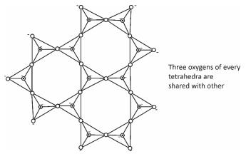
In pyrosilicates, there is only one shared oxygen, in linear chain silicates, two oxygen per tetrahedral are shared while in three-dimensional silicates, all four oxygen's are shared.
